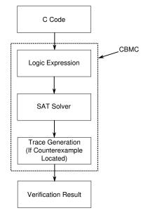
Figure 12.2: CBMC Processing Flow
