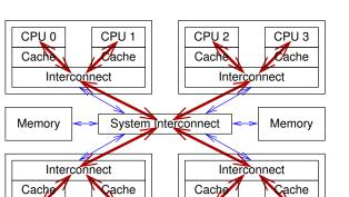
Figure E.1: Data Flow For Global Combining-Tree Atomic Increment
