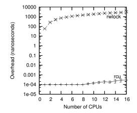
Figure 9.17: Performance Advantage of RCU Over Reader-Writer Locking
