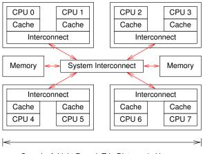
Speed–of–Light Round–Trip Distance in Vacuum for 1.8 GHz Clock Period (8 cm)
