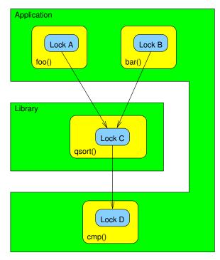
Figure 7.6: Layered Locking Hierarchy for qsort()
