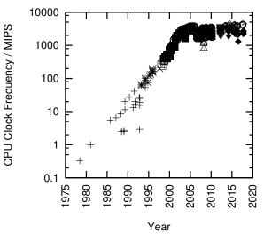
Figure 6.11: MIPS/Clock-Frequency Trend for Intel CPUs
