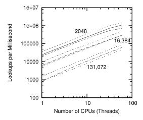
Figure 10.17: Overhead of Resizing Hash Tables
