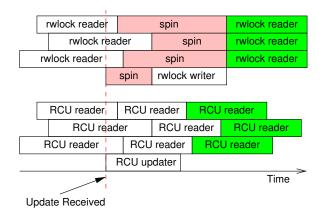
Figure 9.20: Response Time of RCU vs. Reader-Writer Locking
