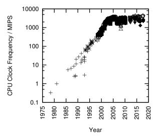
Figure 2.1: MIPS/Clock-Frequency Trend for Intel CPUs
