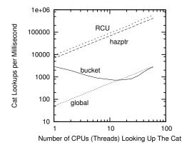
**Figure 10.8:** Read-Side Cat-Only RCU-Protected Hash-Table Performance For Schrödinger's Zoo at 60 CPUs
