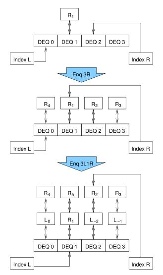
Figure 6.8: Hashed Double-Ended Queue After Insertions
