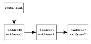
Figure 9.1: Pre-BSD Packet Routing List
