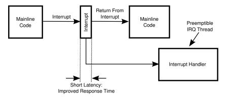
Figure 14.13: Threaded Interrupt Handler
