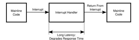
Figure 14.12: Non-Threaded Interrupt Handler
