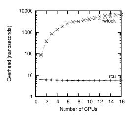
Figure 9.18: Performance Advantage of Preemptible RCU Over Reader-Writer Locking
