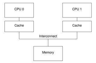
Figure C.1: Modern Computer System Cache Structure
