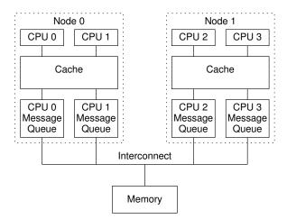
Figure C.8: Example Ordering-Hostile Architecture
