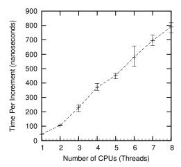
Figure 5.1: Atomic Increment Scalability on Nehalem
