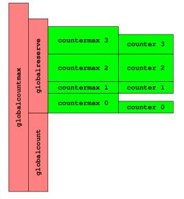
Figure 5.5: Simple Limit Counter Variable Relationships
