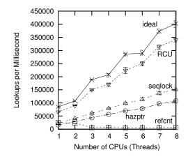
Figure 9.15: Pre-BSD Routing Table Protected by RCU
