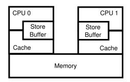
Figure 15.1: System Architecture With Store Buffers
