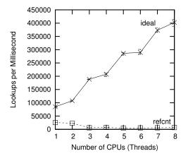
Figure 9.2: Pre-BSD Routing Table Protected by Reference Counting
